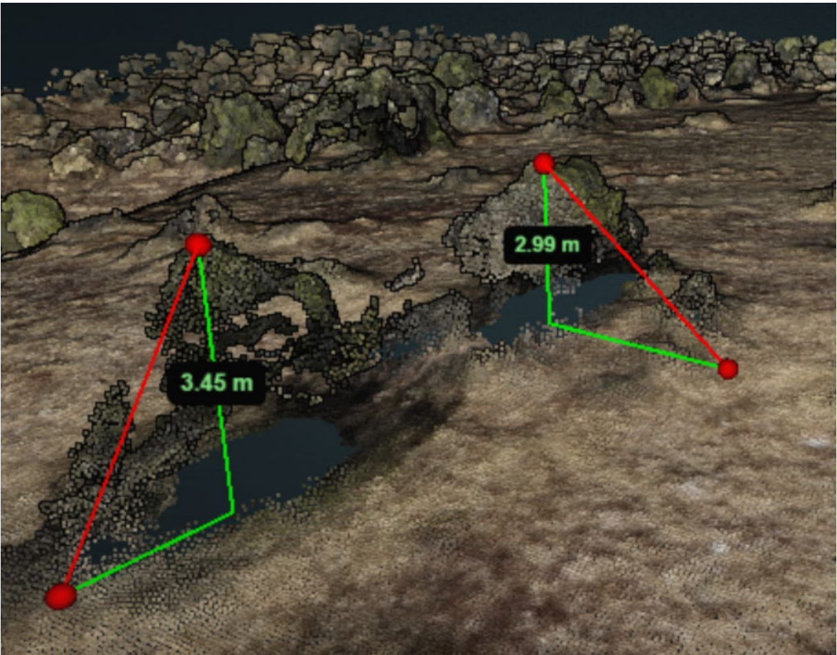
Example: measuring vegetation heights using drones.
